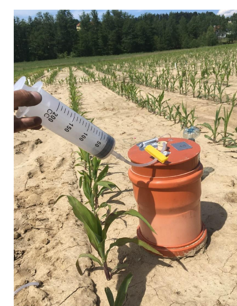
Fig. 1: Soil greenhouse gas emission measurement
